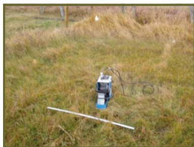
Taking soil water measurements at Souris using a neutron probe.
